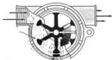
Hall-Effect-Sensor sends a voltage pulse with each pass of magnetic field
